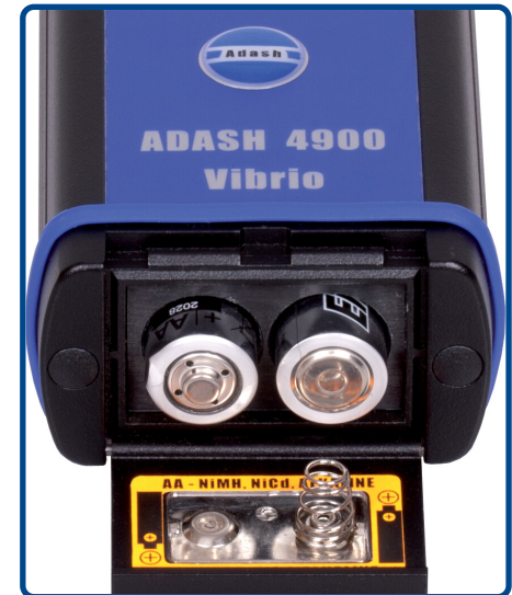
Placement of batteries
