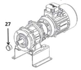
Heat new friction ring at 110 ±10°C / 230 ±50°F.
