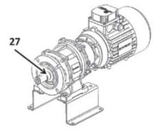
Let friction ring cool down before carrying on reassembly. Put back the pump body.
