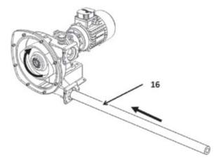
If pump rotates anti-clockwise, suction is on the top port :
