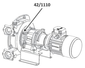
Refit rotor in the pump (see § ROTOR REMOVAL), refit hose (see § HOSE REPLACEMENT) and fill the pump with lubricant (see § LUBRICANT REPLACEMENT).
