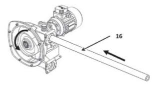
Rotate the pump intermittently until the hose 16 is completely inserted in the body and show equal lengths outside the body on both ports :
