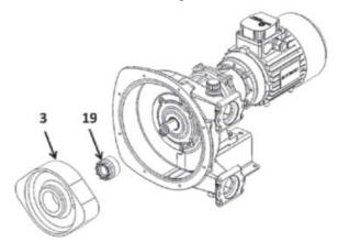
Position rotor 3 to have distance B between rotor outer edge and casing 1 back wall.
