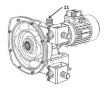
Fill the pump with corresponding volume of lubricant : HD10 .....0,2 I. (0,052 gal.) HD15 - HD20 .....0,6 I. (0,185 gal.)
