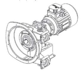
Put back nuts 42 and their washers 1110 and tighten them. **Tightening torque 19 Nm**.
