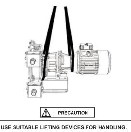
Pass a strap between pump body and gear reducer. Pass another one between gear reducer and motor and put all straps on a common hook.
