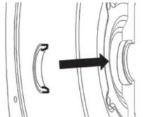
If necessary to replace friction ring 27, use a mallet and a chisel, to break and remove friction ring 27.
