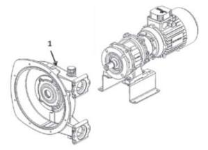
Remove shaft seal 26 from pump body. Put new shaft seal 26 in pump body.
