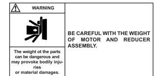
Using appropriate lifting device, lift motor and reducer assembly.
