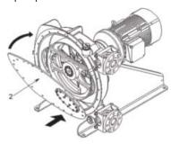
Screw and tighten screws 33 and their washers 34, starting by top ones to secure cover assembly.
