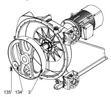
Position rotor 3 to have distance B between rotor outer edge and casing 1 back wall.
