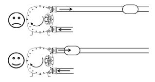
Change pumping set or pump ports position rather than multiplying pipe bends.
