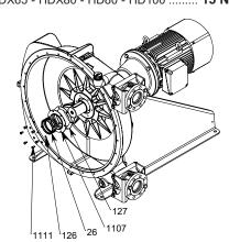
Refit rotor in the pump (see § ROTOR REMOVAL), refit hose (see § Hose REPLACEMENT) and fill the pump with lubricant (see § LUBRICANT REPLACEMENT).
