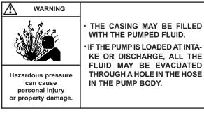
When the hose breaks, there is a risk that the lubricant may be contaminated by the pumped liquid.
