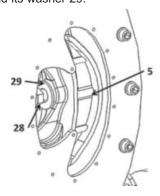
Pull the shoe 5 and its shim(s) 4, first in the radial direction to let pin come out of the rotor then out of the pump.
