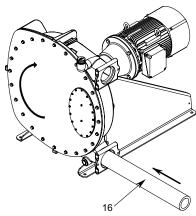
If pump rotates anti-clockwise, suction is on the top port :
