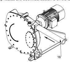
Rotate the pump intermittently until the hose 16 is completely inserted in the body and show equal lengths outside the body on both ports:
