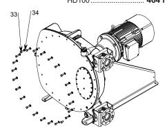
Fit hose in (see § HOSE REPLACEMENT) and fill the pump with lubricant (see § LUBRICANT REPLACEMENT).
