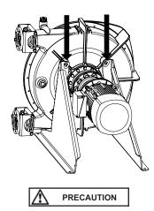
USE SUITABLE LIFTING DEVICES FOR HANDLING. USE THE LIFTING RINGS PROVIDED.
