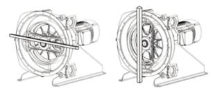
Put cover gasket 10 in pump body, starting at the top. Make sure that the two ends of gasket are firmly in contact.
