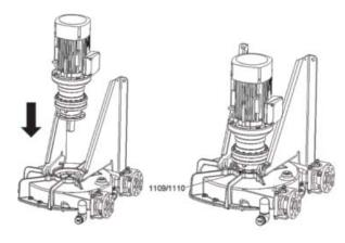
Put back studs 41 with their nuts 42 (HD50 - HD65) or screws 1109 with their washers 1110 (HDX65 - HDX80 -HD80) and tighten them.
