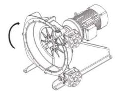
Assemble shaft seals 26 in seal holder 1107.
