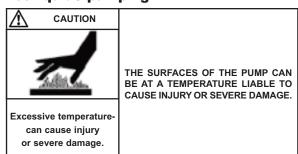
When pumping products at high temperatures, take care when starting the pump for the first time, tighten the bolts to compensate for expansion effects.
