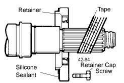
Figure 71 - Remove Bearing Retainers
