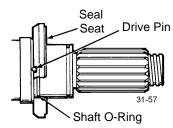
Figure 56 - Install O-Rings
