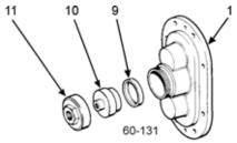
Figure 103 - Pneumatic Vented Cover
