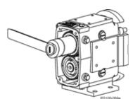
Figure 92 - Install Gear Locknuts
