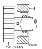
Figure 95 - Orientation of Oil Seal
