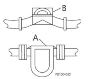
A. Strainer B. Magnetic Trap Figure 15 - Inline Strainers and Traps
