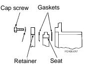
Figure 62 - Install Seal Components
