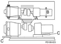
Figure 20 - Check Parallel Alignment
