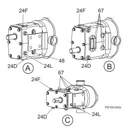
Figure 23 - Lubrication Points
