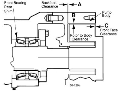
Figure 94 - Clearance Measurements
