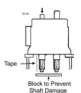
Figure 73 - Press Shafts from Gear Case
