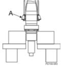
Figure 79 - Press Lower Cone onto Shaft
