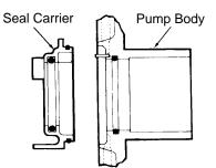
Figure 44 - Assemble Carriers into Body
