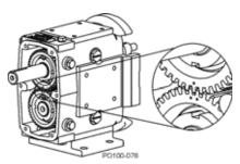
Figure 90 - Timing Gear Marks
