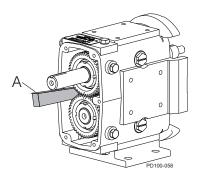
Figure 70 - Block Shaft Rotation
