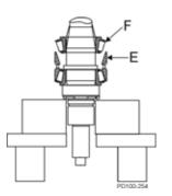
Figure 81 - Install Upper Cup & Upper Cone
