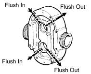
Figure 109 - Flushing Connections
