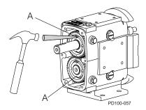
Figure 69 - Straighten Lock Tab
