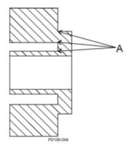
Figure 30 - Rotor Stress Points
