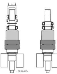
Figure 83 - Rear Tapered Roller Bearing Assembly
