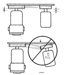
Use a straight edge to visually check the belt or chain alignment. Keep the shaft distance to a minimum (Figure 21, item A).
