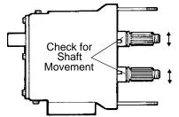
Figure 28 - Bearing Deflection Check
