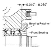
Figure 86 - Bearing Retainer Clearance
