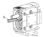
Figure 91 - Block Shaft Rotation
