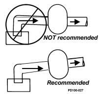
Figure 10 - Correct Piping to Prevent Inlet Air Pockets
