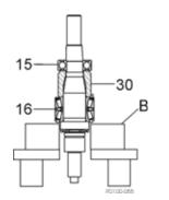
Figure 76 - Remove Bearings from Shaft
