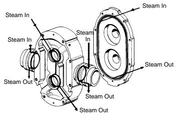
Figure 110 - Flushing Connections - Aseptic Series
