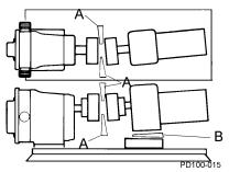
Figure 19 - Check Angular Alignment
