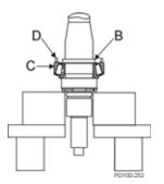
Figure 80 - Install Inner & Outer Spacer, Lower Cup
