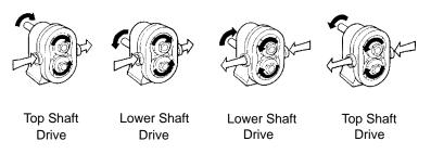
Figure 22 - Direction of Drive Rotation
