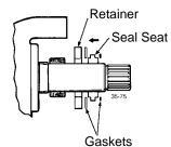
Figure 65 - Install Inner Seal
