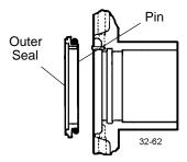
Figure 53 - Insert Seal Assembly
