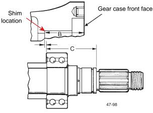
Figure 85 - Measure B and C
