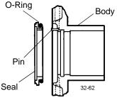
Figure 57 - Install Seal Seats
