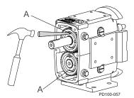
Figure 93 - Bend Locking Tab
