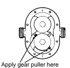
Figure 34 - Apply Gear Puller
