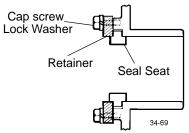
Figure 60 - Remove Seal Seat Retainer
