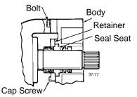
Figure 67 - Position Seal Retainer
