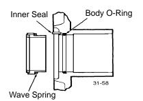
Figure 49 - Assemble Wave Spring
