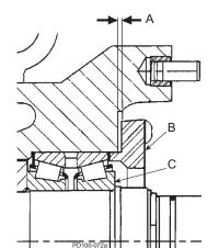
Figure 209 - Bearing Retainer Clearance
