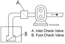
Figure 12 - Inlet Check Valve
