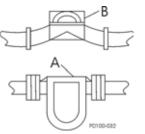
A. Strainer B. Magnetic Trap Figure 19 - Inline Strainers and Traps
