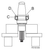
Figure 203 - Install Inner & Outer Spacer and Lower Cup
