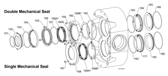
Figure 222 - Mechanical Seals, U3 pumps 180-U3 and larger
