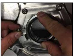
Figure 99 - Install seal retaining bolts
