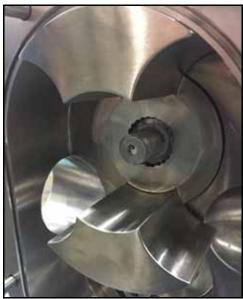
Figure 181 - Rotor installed
