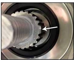
Figure 179 - Timing spline of shaft
