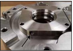
Figure 160 - Flush hole location
