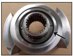
Figure 173 - Sleeve front O-ring
