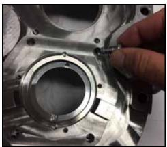
Figure 91 - Seal housing bolts
