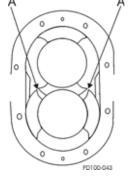
Figure 31 - Rotor to Rotor Tip Clearance
