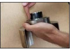
Figure 177 - Lubricate seal sleeve
