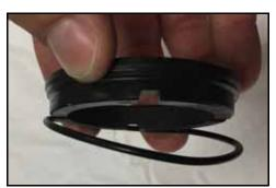
Figure 44 - Stationary Seal O-ring
