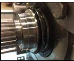
Figure 107 - O-ring installed
