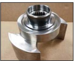
Figure 176 - Seal sleeve installed
