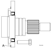
Figure 196 - Remove Sealant from Retainer
