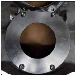
Figure 68 - Seal housing installed
