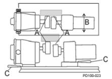
Figure 27 - Check Parallel Alignment
