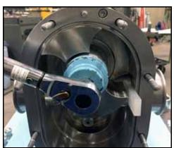
Figure 38 - Remove Rotor Nut
