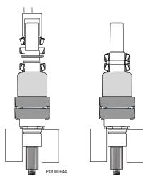
Figure 206 - Rear Tapered Roller Bearing Assembly
