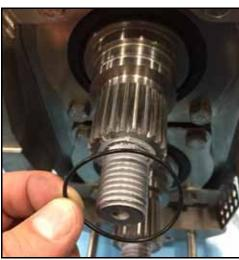
Figure 102 - Install O-ring
