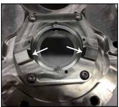
Figure 92 - Seal housing installed
