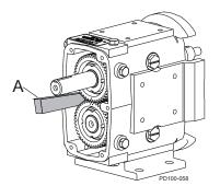
Figure 215 - Block Shaft Rotation
