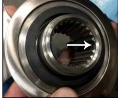
Figure 178 - Timing spline of rotor
