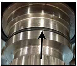
Figure 123 - O-ring installed
