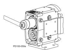
Figure 216 - Install Gear Locknuts
