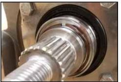
Figure 167 - Install wave spring
