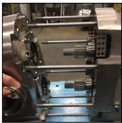
Figure 151 - Remove pump body
