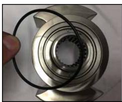
Figure 42 - Remove seal O-ring
