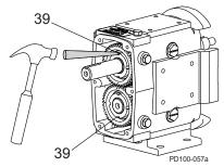
Figure 217 - Bend Locking Tab
