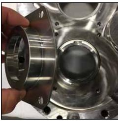
Figure 48 - Remove seal housing
