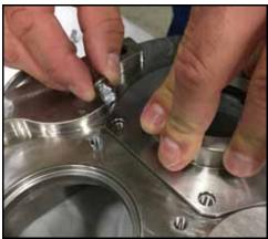
Figure 61 - Install seal housing bolts
