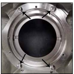
Figure 115 - Seal housing bolts
