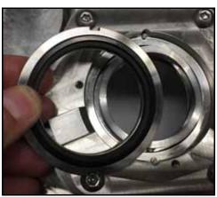
Figure 74 - Remove stationary seal
