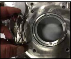
Figure 50 - Remove wave spring
