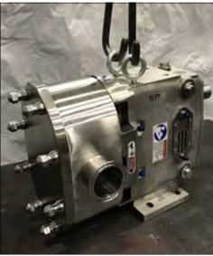
Figure 3 - Lifting location
