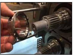
Figure 104 - Install adjusting ring
