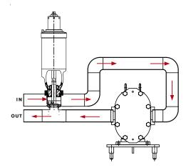
Figure 17 - WR61C Air-to-Raise Valve with Adjustable-Spring Actuator
