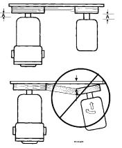
Figure 28 - Aligning Belt and Chain Drives
