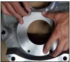
Figure 67 - Install seal housing bolts
