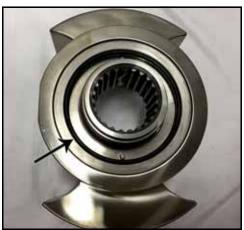
Figure 139 - Seal O-ring installed
