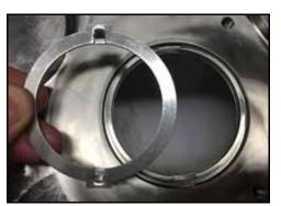
Figure 56 - Install drive ring
