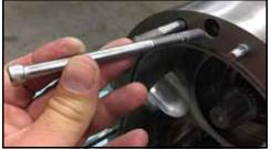
Figure 150 - Remove body retaining screws
