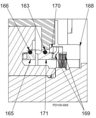
Figure 224 - U3 Single Mechanical Seal
