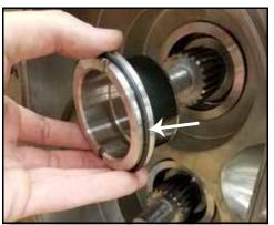
Figure 145 - Remove sleeve, O-ring
