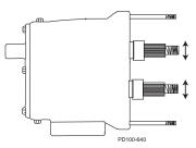
Figure 34 - Bearing Deflection Check
