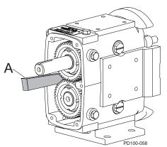
Figure 194 - Block Shaft Rotation
