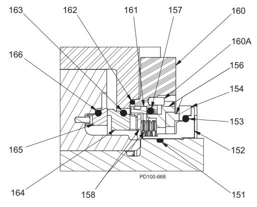
Figure 225 - U3 Double Mechanical Seal
