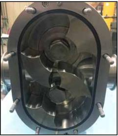
Figure 188 - Cover gasket installed
