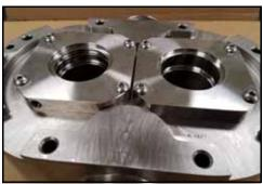
Figure 162 - Seal housings installed
