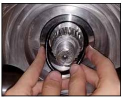
Figure 171 - Install seal O-ring
