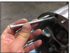
Figure 170 - Install body retaining screws
