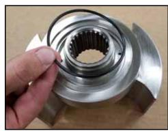
Figure 172 - Install sleeve front O-ring
