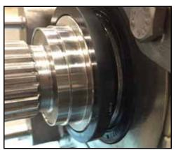
Figure 109 - Rotary seal installed
