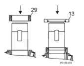
Figure 213 - Install Rear Seal
