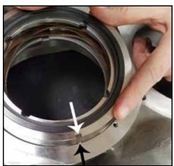
Figure 119 - Install flush-side stationary seal
