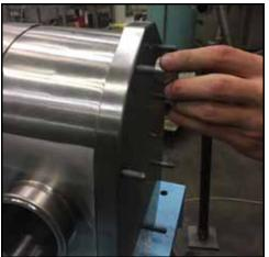
Figure 190 - Install cover nuts
