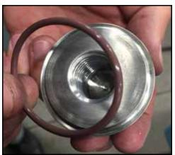
Figure 182 - Install O-ring
