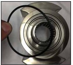
Figure 138 - Install seal O-ring
