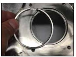
Figure 82 - Remove shaft ring
