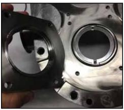
Figure 90 - Install seal housing
