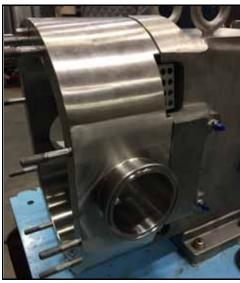
Figure 131 - Pump body installed
