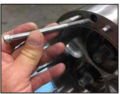
Figure 132 - Install body retaining screws
