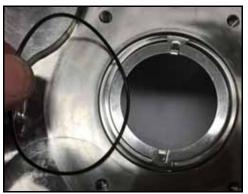
Figure 79 - Remove seal housing Oring
