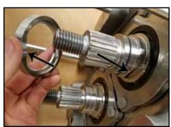
Figure 165 - Install seal seat
