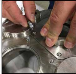
Figure 47 - Remove seal housing bolts
