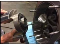
Figure 180 - Push rotor on shaft
