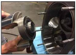
Figure 40 - Remove rotor
