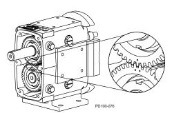
Figure 214 - Timing Gear Marks
