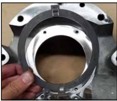
Figure 63 - Install drive ring
