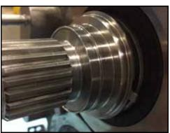
Figure 125 - Adjusting ring installed
