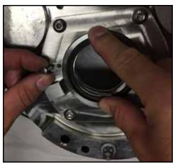
Figure 73 - Remove seal retaining bolts
