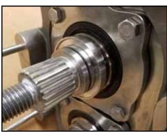
Figure 166 - Seal seat installed
