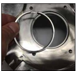
Figure 52 - Remove shaft ring
