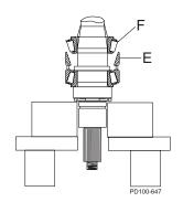
Figure 204 - Install Upper Cup & Upper Cone
