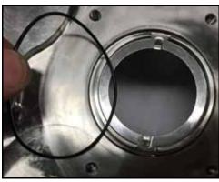
Figure 88 - Install seal housing O-ring
