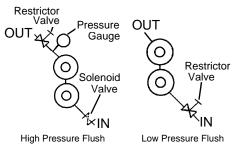
Figure 23 - Flush Piping Setup
