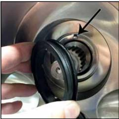
Figure 135 - Install stationary seal
