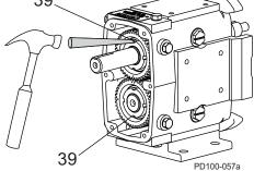
Figure 193 - Straighten Lock Tab on Lock Washers
