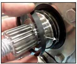
Figure 128 - Install flush-side rotary seal
