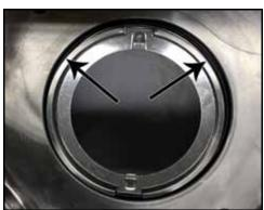
Figure 89 - Seal housing O-ring installed
