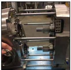
Figure 46 - Remove pump body
