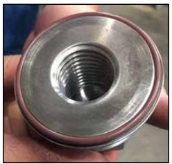
Figure 183 - O-ring installed
