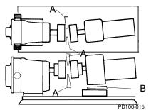
Figure 26 - Check Angular Alignment
