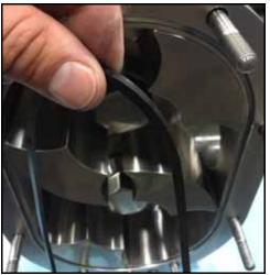
Figure 187 - Install cover gasket
