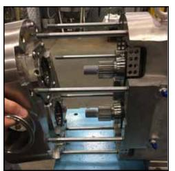
Figure 168 - Install pump body
