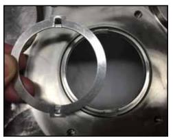
Figure 86 - Install drive ring
