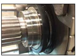
Figure 129 - Rotary seal installed
