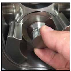
Figure 184 - Install rotor nut
