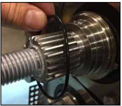
Figure 106 - Install O-ring
