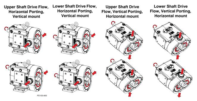
Figure 29 - Pump Rotation (Liquid End Shown)
