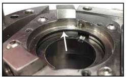
Figure 76 - Seal O-ring location
