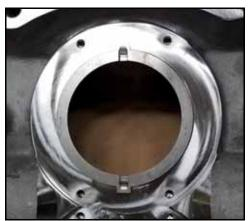
Figure 64 - Drive ring installed
