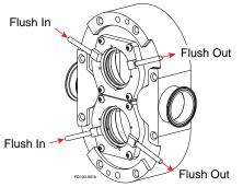
Figure 22 - Flush Piping - Liquid, Steam, Steam Condensate
