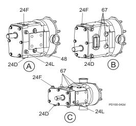
Figure 30 - Lubrication Points
