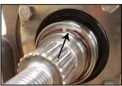
Figure 155 - Remove wave spring
