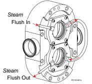
Figure 21 - Flush Piping - Steam
