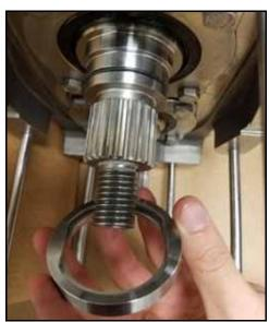
Figure 156 - Remove seal seat
