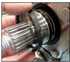
Figure 69 - Remove flush-side rotary seal
