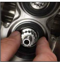
Figure 136 - Push on stationary seal
