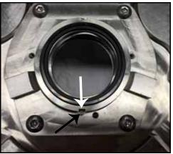
Figure 98 - Flush-side stationary seal installed
