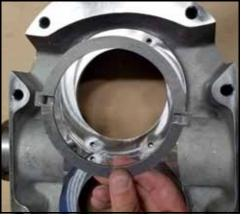
Figure 110 - Install drive ring
