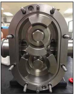
Figure 186 - Rotors installed
