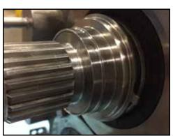
Figure 105 - Adjusting ring installed
