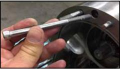
Figure 45 - Remove body retaining screws
