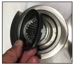
Figure 41 - Remove rotary seal
