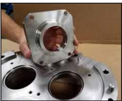
Figure 159 - Line up bolt holes
