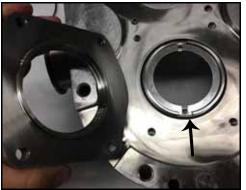
Figure 78 - Remove seal housing
