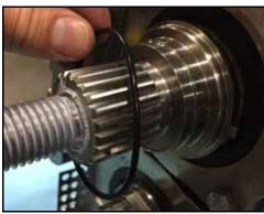
Figure 126 - Install O-ring
