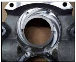
Figure 111 - Drive ring installed
