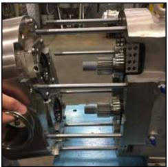
Figure 130 - Install pump body
