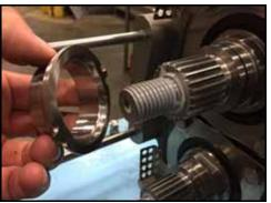
Figure 71 - Remove adjusting ring
