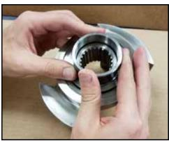
Figure 175 - Press sleeve into place
