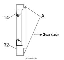
Figure 212 - Install Bearing Retainer
