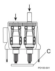
Figure 197 - Press Shafts from Gear Case
