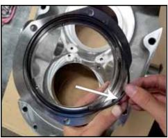
Figure 112 - Install seal housing Oring
