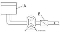
A. Closed Tank - produces vacuum on liquid (Low Absolute Pressure)B. Check Valve (outlet)
