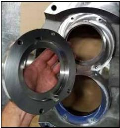
Figure 49 - Remove seal housing
