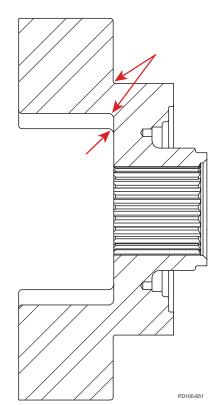
Figure 35 - Rotor Stress Points
