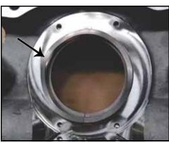
Figure 65 - Wave spring installed
