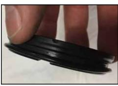
Figure 134 - Seal O-ring installed
