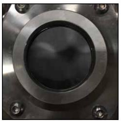
Figure 62 - Seal housing installed
