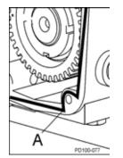
Figure 220 Sealant Placement
