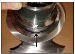
Figure 174 - Line up notch and pin
