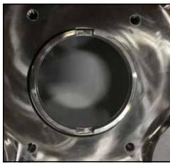
Figure 55 - Ring installed
