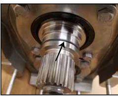
Figure 164 - O-ring installed
