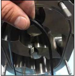
Figure 37 - Remove cover gasket
