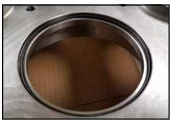
Figure 158 - Seal housing O-ring installed
