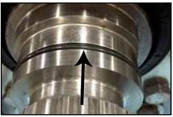
Figure 72 - Adjusting ring O-ring
