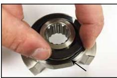
Figure 142 - Seal O-ring pinched
