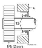
Figure 219 - Orientation of Oil Seal
