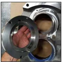
Figure 66 - Install seal housing
