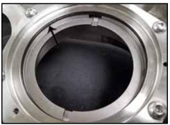
Figure 117 - Seal O-ring location
