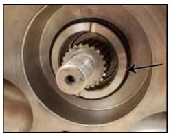
Figure 144 - Sleeve remaining after rotor removal
