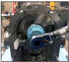
Figure 185 - Torque rotor nut
