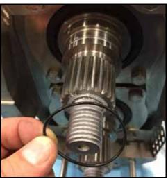
Figure 122 - Install O-ring
