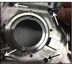
Figure 77 - Seal housing bolts
