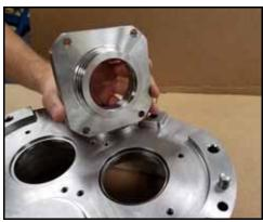
Figure 153 - Remove seal housing
