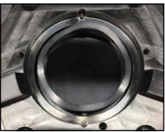
Figure 96 - Wave spring installed
