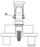
Figure 202 - Press Lower Cone onto Shaft
