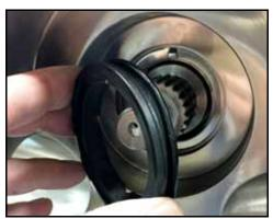
Figure 43 - Remove stationary seal
