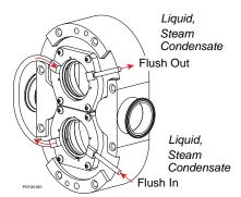
Figure 20 - Flush Piping - Liquid, Steam Condensate
