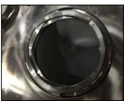
Figure 59 - Wave spring installed
