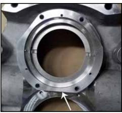
Figure 114 - Seal housing in place
