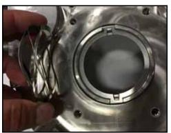
Figure 58 - Install wave spring
