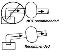
Figure 11 - Piping Slope
