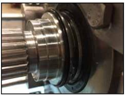
Figure 127 - O-ring installed
