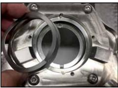
Figure 75 - Remove wave spring
