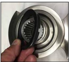
Figure 140 - Install rotary seal
