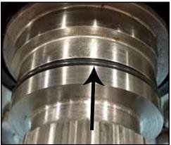
Figure 103 - O-ring installed
