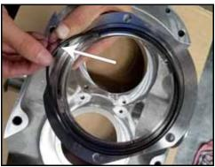
Figure 80 - Remove seal housing Oring
