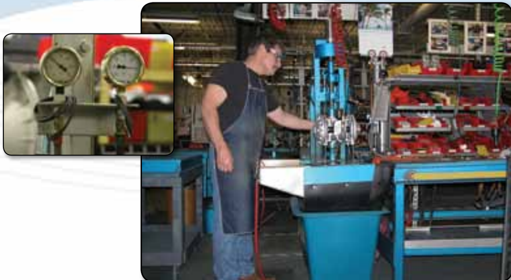
Experienced Warren Rupp assembler monitors pump performance with pressure and vacuum gauges.
