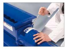
2. The feed chamber is pulled back to allow full access to the pin joint area for removal of any blockages or compressed cake
