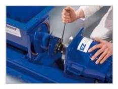
6. Unscrew the rotor from the stator
