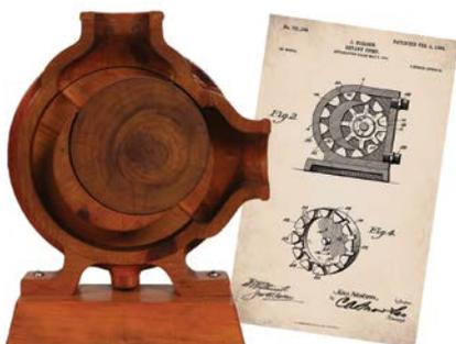
This wooden model was hand carved by Jens Nielsen. Its Gear-Within-A-Gear design was used to solve Nielsen’s water seepage problem and was the foundation on which the Viking Pump Company was founded.
