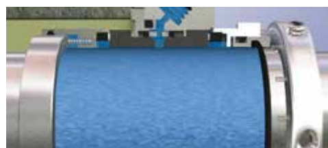
4. Double mechanical seal with cool / clean barrier fluid
