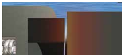
2. Fluid film cooling the seal faces
