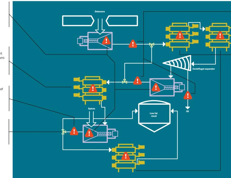
Circumferential piston pump Scraped surface heat exchanger for high efficiency cooling, heating and tempering. It is designed to handle highly viscous fluids or products, which
