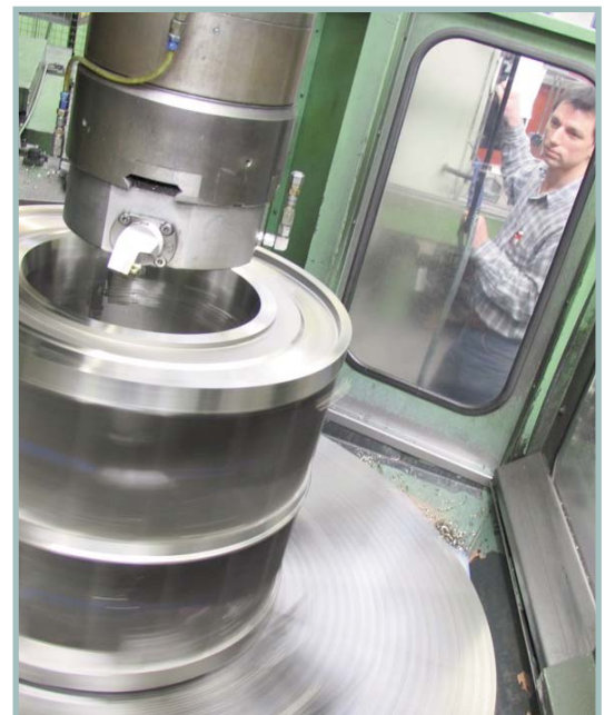
Refinishing of an impeller
