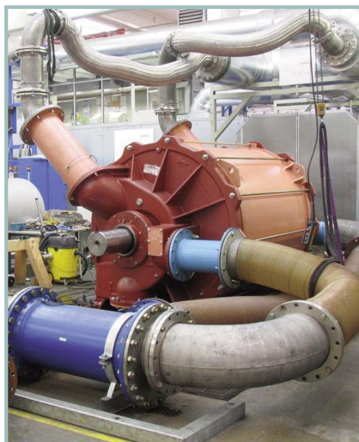
Pump during performance test in the test field
