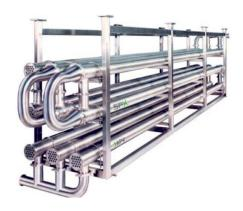
The **Corrugated Quadruple Tube (CQT)** offers significant flexibility in the annulus gap to optimize heat transfer and pressure drop. This feature is critical to heat transfer of laminar and/or non-Newtonian fluids, particularly to product-to-product regeneration.
