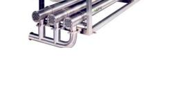
The Corugated Quadruple Tube (CQT) offers significant flexibility in the annulus gap to optimize heat transfer and pressure drop. This feature is critical to heat transfer of laminar and/or non-Newtonian fluids, particularly to product-to-product regeneration.
